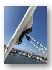
On this yacht you have self tacking jib, which means when you want to open the genoa you must release the genoa sheet and to take out the genoa furling. This procedure must be simultaneously. If you want to close the genoa sail you must release the furling rope and to pull the genoa sheet. This procedure must be simultaneously.
