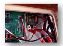
At the image indicates fuse of the Windlass. In case the fuse has fallen, you will see the yellow plastic protruding at the position zero (0), with the use of your hand (fingers) you press the yellow plastic down so that it reaches at the position one (1). Then does an operation test to find out if everything is working properly.
