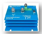
The Smart Battery Protect disconnects the battery from non-essential loads before it is completely discharged (which would damage the service batteries) or before it has insufficient power left to crank the service batteries. When using Bluetooth to program the Smart Battery Protect any required engage/disengage levels can be set. <a href="https://www.victronenergy.com/panel-systems-remote-monitoring/victronconnect">https://www.victronenergy.com/panel-systems-remote-monitoring/victronconnect</a>
