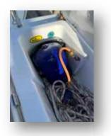
For more safety if you want to close all system of gas you need to go outside at the starboard side and to open the locker. There, you will find the bottle gas. If you turn the valve clockwise you open the gas system and when you turn the valve from the other direction you close the gas system.
