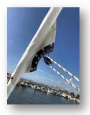
On this yacht you have self tacking genoa, which means when you want to open the genoa you must release the genoa sheet and to take out the genoa furling. This procedure must be simultaneously. If you want to close the genoa sail you must release the furling rope and to pull the genoa sheet. This procedure must be simultaneously.
