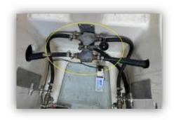
This yacht has two diesel tanks. When you want to change the diesel tank you need to go in front of the stairs and to open the cup. When the valve is on the right you take diesel from the  $1^{\rm st}$  diesel tank and when the valve is go at the stern right side on the left you take diesel from the  $2^{\rm nd}$  diesel tank.
