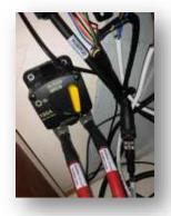
At the image indicates fuse of the Windlass. In case the fuse has fallen, you will see the yellow plastic protruding at the position zero (0), with the use of your hand (fingers) you press the yellow plastic down so that it reaches at the position one (1). Then does an operation test to find out if everything is working properly. You will find it under of the chart table.
