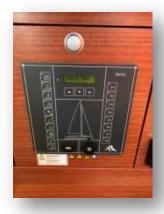
These devices can control the windlass, thrusters, navigation lights, alarms, video surveillance systems, windshield wipers, engines, fuel, water and oil levels, generators and other equipment.
